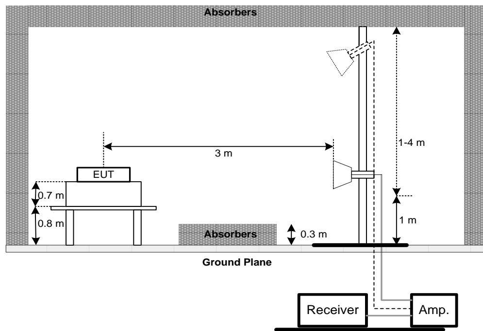
(C) For radiated emissions below 30MHz
