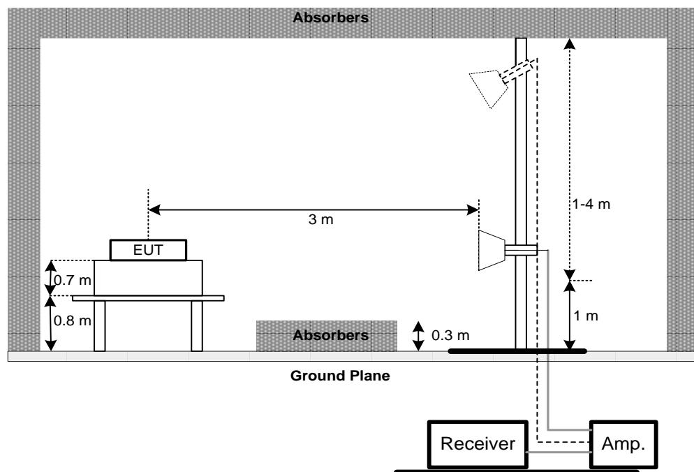
(C) For Radiated Emissions Below 30MHz
