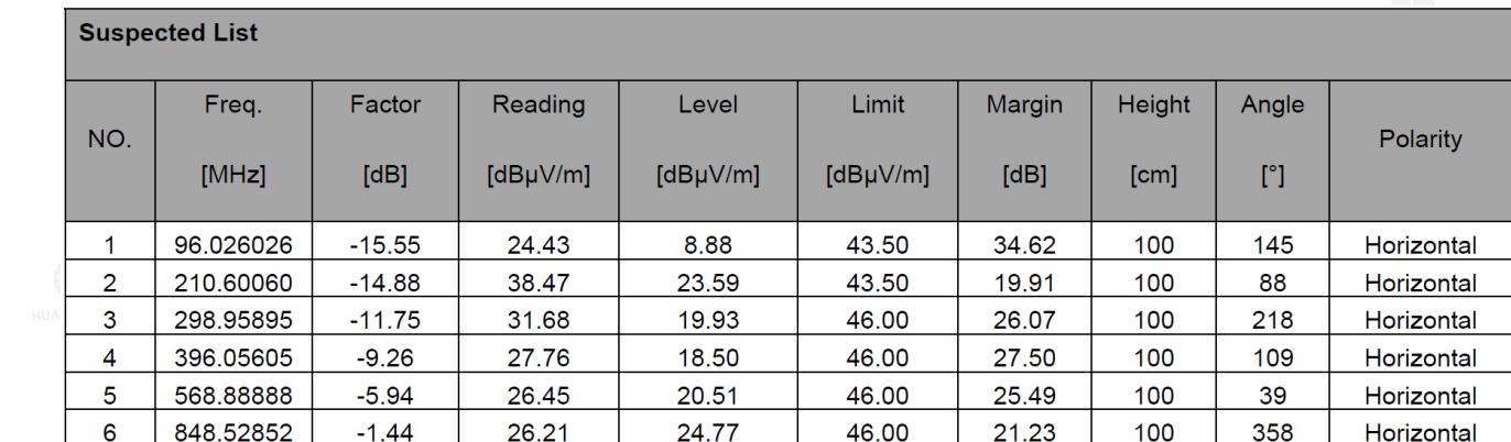
Remark: Factor = Cable loss + Antenna factor + Attenuator – Preamplifier; Level = Reading + Factor;
