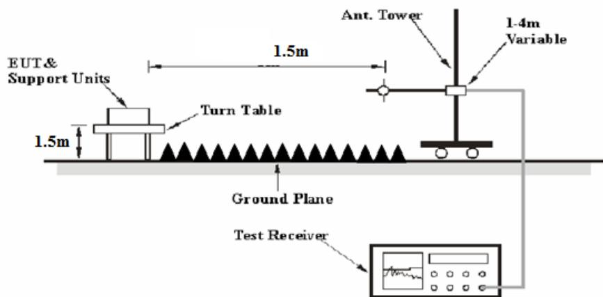
The radiated emission tests were performed in the 3 meters chamber test site, using the setup accordance with the ANSI C63.10-2013. The specification used was the FCC 15.209, FCC 15.249 and RSS-210, RSS-Gen limits.
