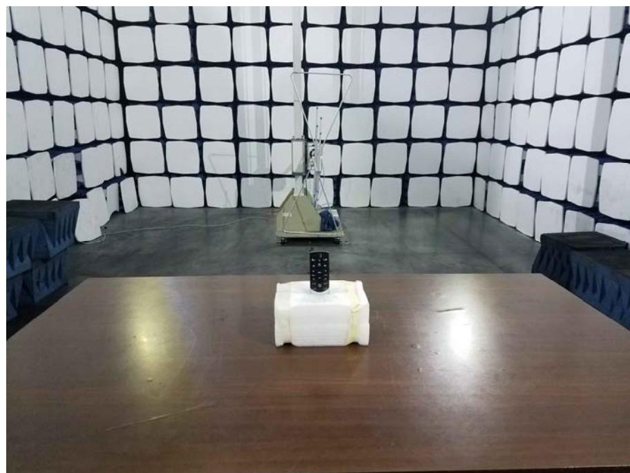
**Radiation Emission Test Setup (Above 1GHz)**
