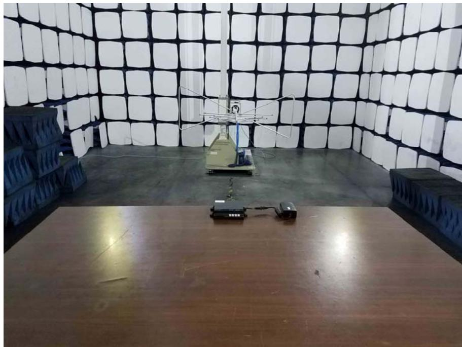
**Radiation Emission Test Setup (Above 1GHz)**
