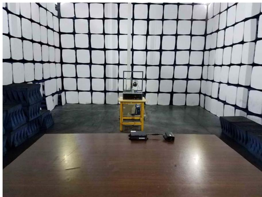
**Radiation Emission Test Setup (30MHz to 1GHz)**
