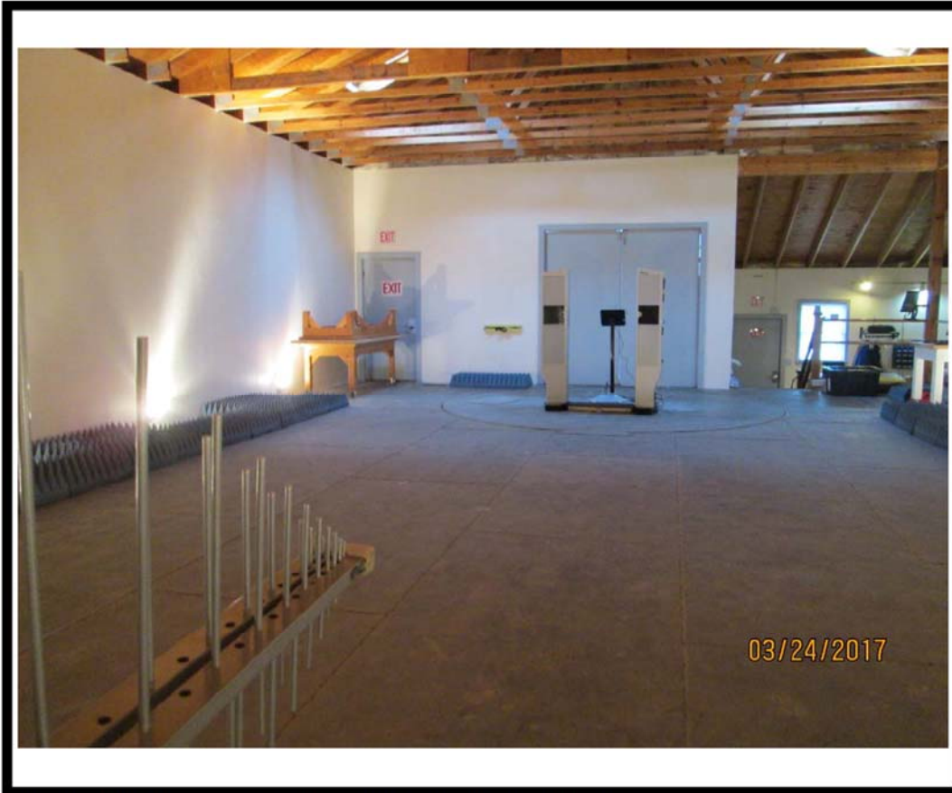
Photograph Description: Radiated set-up – 30MHz through 1GHz
