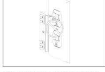
DO NOT plug the rear plate into an outlet by itself. You run the risk of electric shock. If you accidentally plug in the rear plate by itself, turn off the circuit breaker servicing the outlet before attempting to remove the rear plate.
