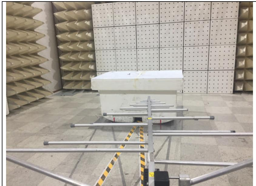
**3. Photo of Radiated Spurious Emission Test (Above 1 GHz)**
