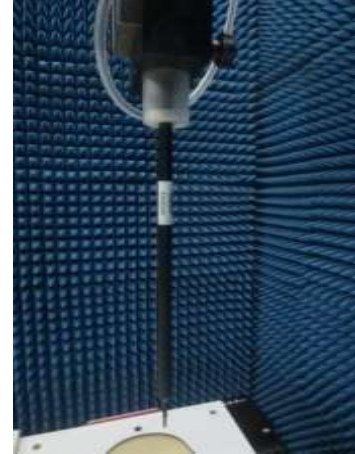
Fig. 8.2 Photo of E-Field Probe
