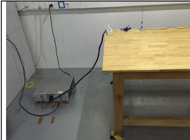
Conducted Emissions Test Setup Front View
