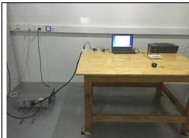
Conducted Emissions Test Setup – Front View
