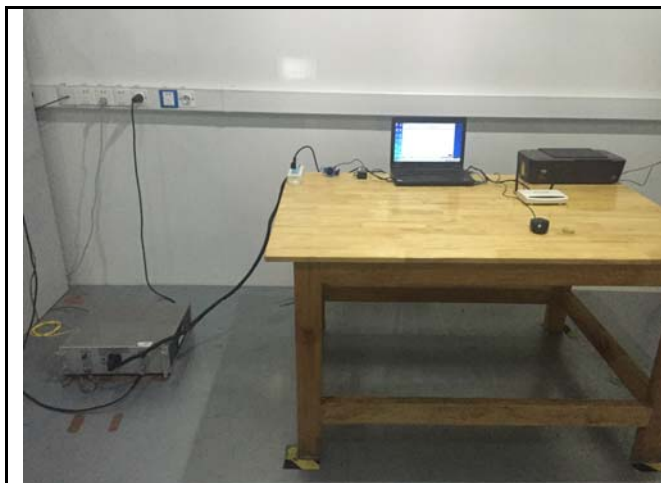
Conducted Emissions Test Setup – Front View
