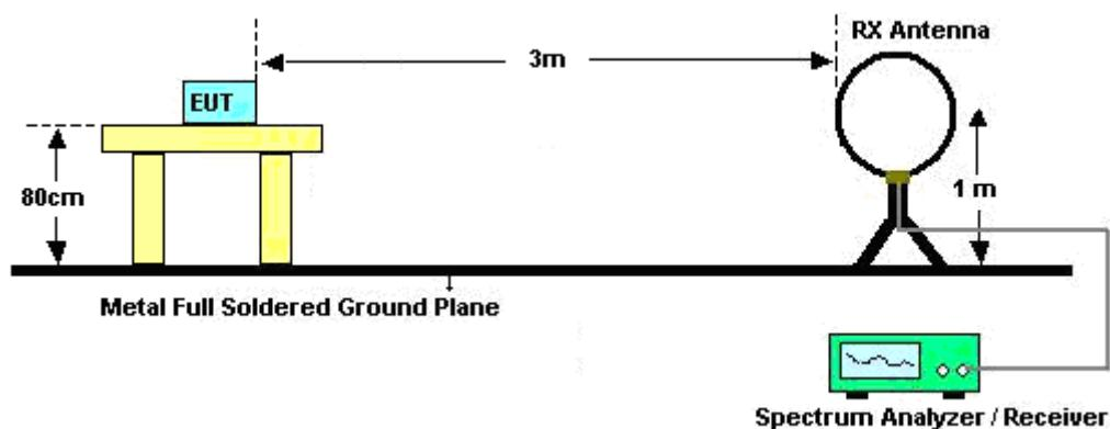
For radiated emissions from 30MHz to 1GHz
