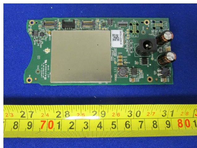
Radio Board with Shielding – Top View
