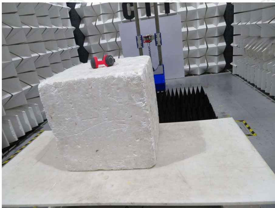
Radiated spurious emission Test Setup-3(Above 1GHz)
