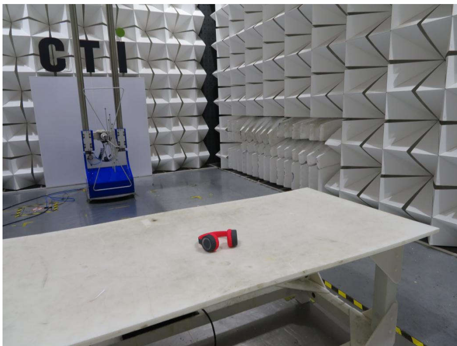
Radiated spurious emission Test Setup-2(30MHz - 1GHz)
