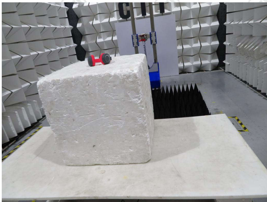
Radiated spurious emission Test Setup-3(Above 1GHz)
