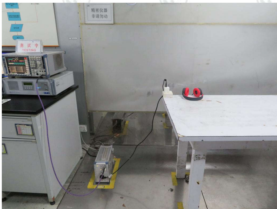
Conducted Emissions Test Setup
