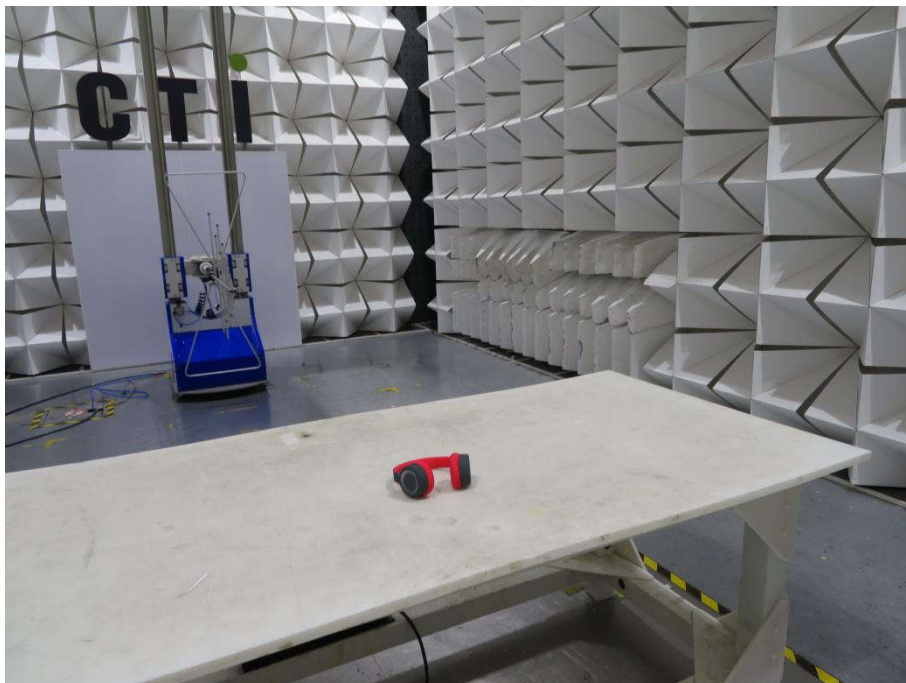
Radiated spurious emission Test Setup-2(30MHz-1GHz)
