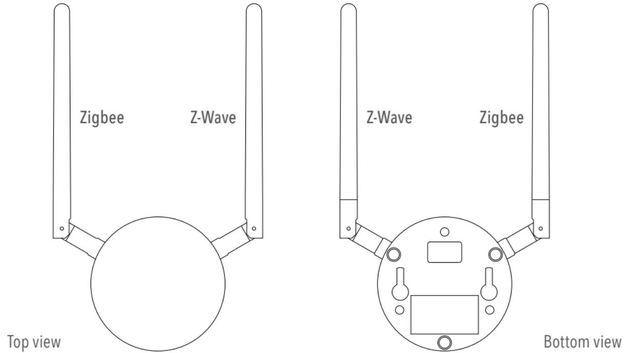
To achieve the best radio performance, make sure to always position antennas vertically and far from metal parts and cables.
