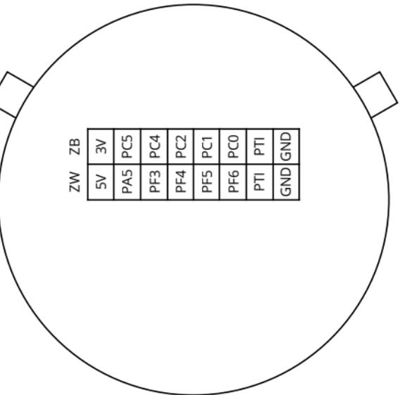
Pins in the ZB row (except for 3V and GND pins) are pins of the Zigbee/Thread/BLE EFR32MG21 chip.
