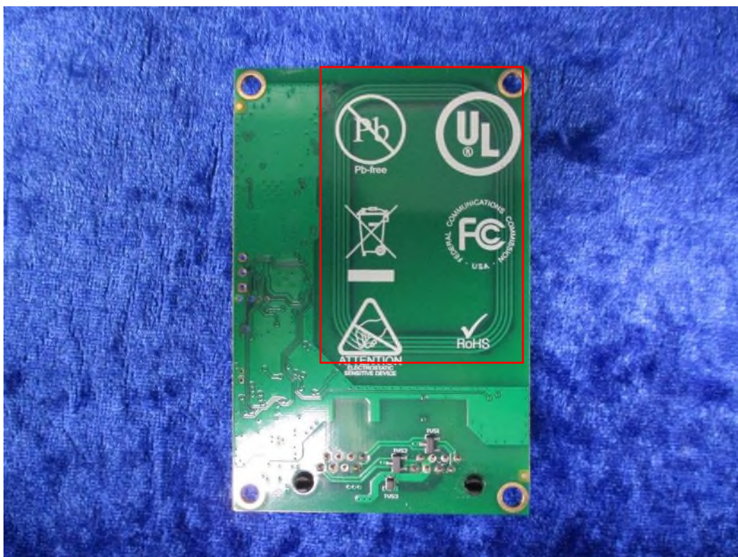
Integral antenna (Outlined in red) this is the same for both of the supplied boards.
