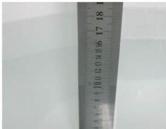
Liquid Height for Body SAR
