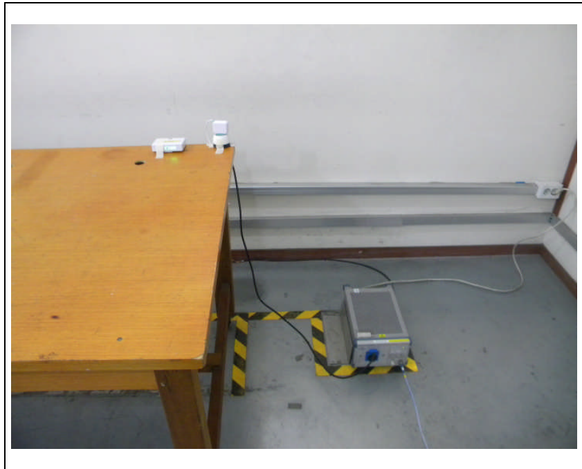
Photo of AC Power line emission Test
