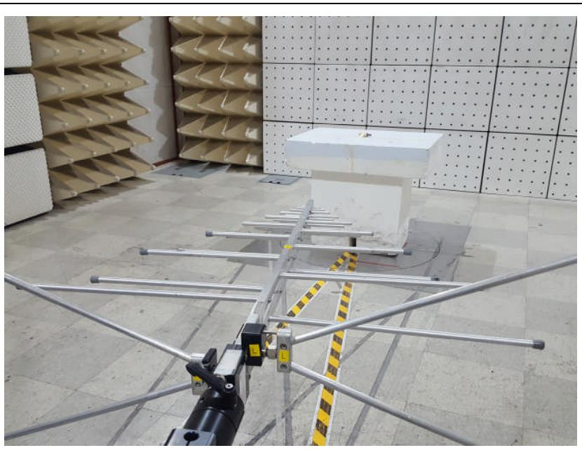
**B. Photo of Radiated Spurious Emission Test (Above 1 GHz)**
