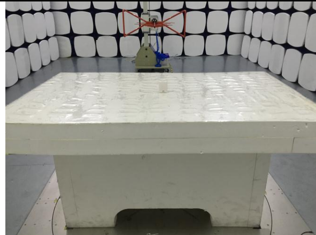
Radiated Spurious Emissions Test Setup Below 1GHz
