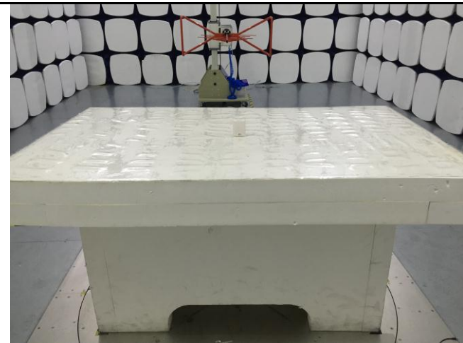
Radiated Spurious Emissions Test Setup Below 1GHz
