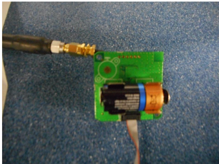
Figure 7: RF Output Power and Occupied Bandwidth Conducted Measurements (close-up views) Test Setup
