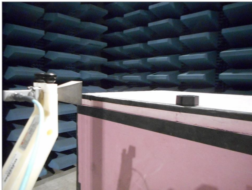
Figure 5: Radiated Emissions (frequency range: 18GHz ↔ 26.5GHz) Test Setup
