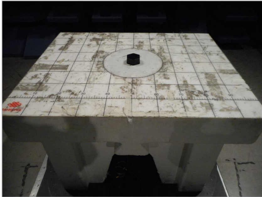
Figure 3: Radiated Emissions (close-up view) Test Setup
