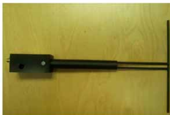
Figure 1 – MVG COMOSAR Validation Dipole
