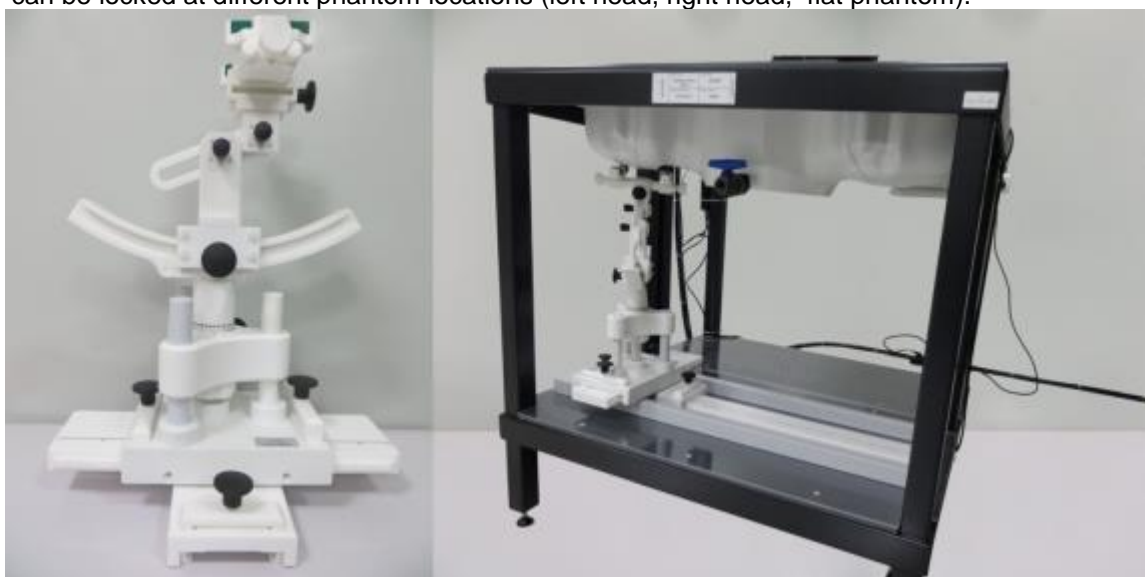
Device holder supplied by SATIMO
