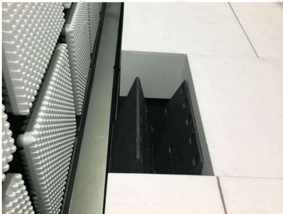
Radiated spurious emission Test Setup-7 (Above 1GHz) There are absorbing materials under the ground.
