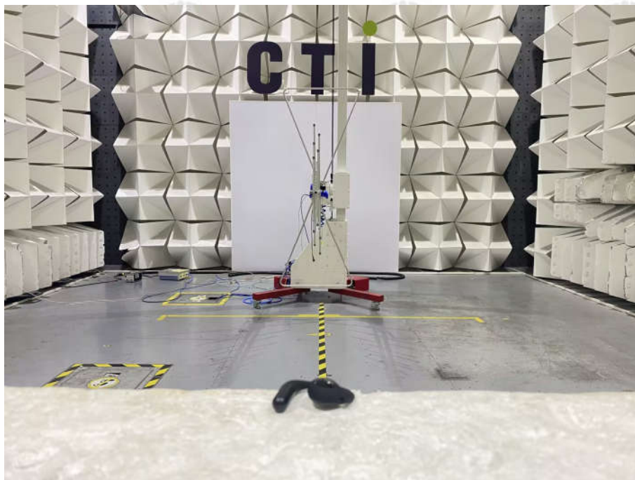
Radiated spurious emission Test Setup-5 Right ear(Below 1GHz) close up
