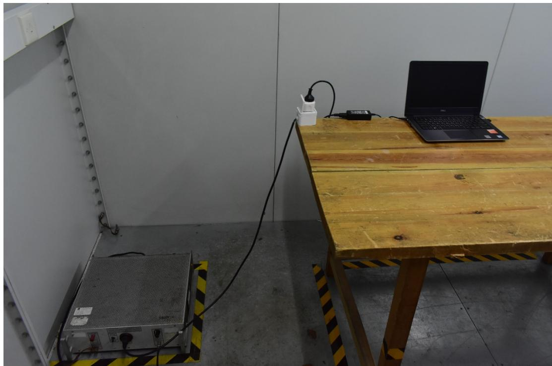
**2. Conducted emission main's port side view**
