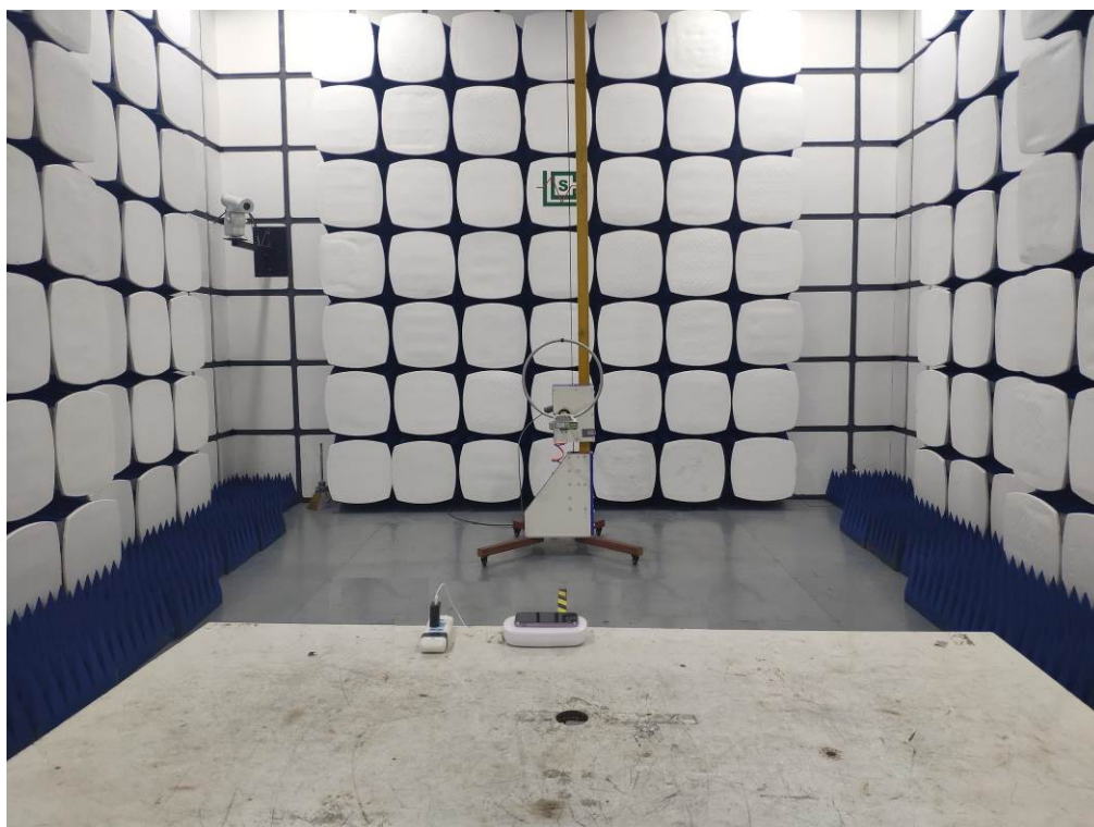
Radiated Emission below 30MHz-AC adapter charge mode
