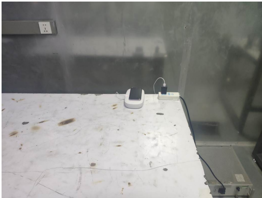
Conducted Emission-AC adapter charge mode
