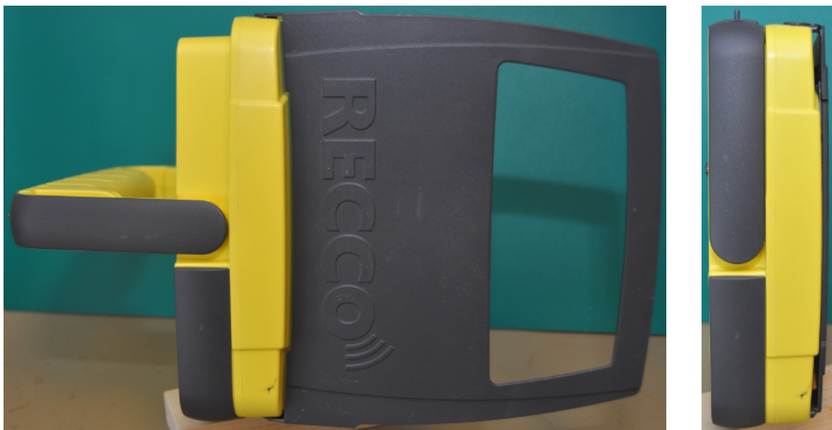
Figure 6: Recco detector top view, antenna and handle opened(left)/closed(right)
