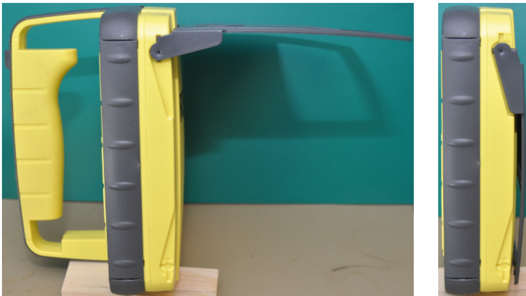
Figure 4: Recco detector left view, antenna and handle opened(left)/closed(right)
