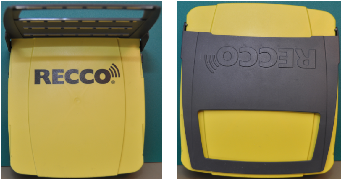
Figure 2: Recco detector front view, antenna opened(left)/closed(right)
