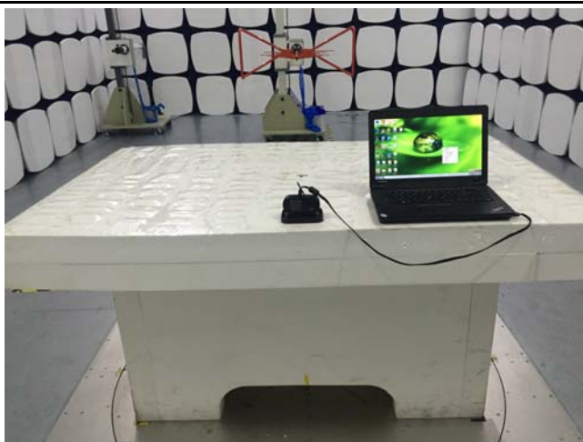
Conducted Emissions Test Setup Front View
