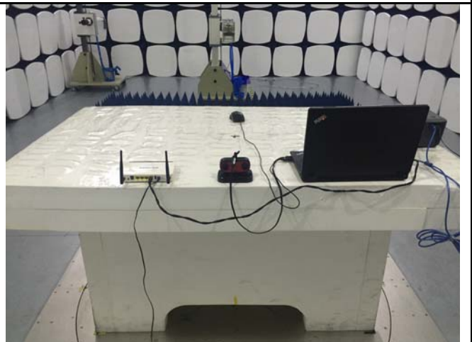
Radiated Emissions Test Setup Above 1GHz
