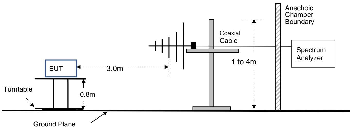
**Radiated Emissions Test Setup for Frequencies over 1000MHz (Side View)**
