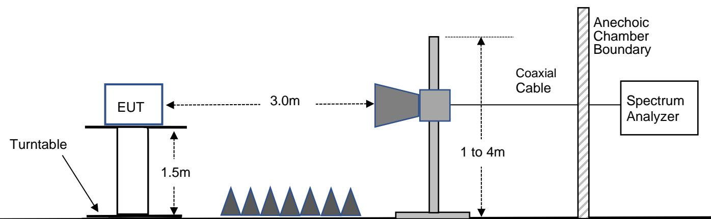
Receive mode used an 80 cm high test stand and transmit mode used an 150 cm test stand.
