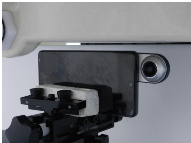
Left side with 10 mm separation distance (Phone with Camera)
