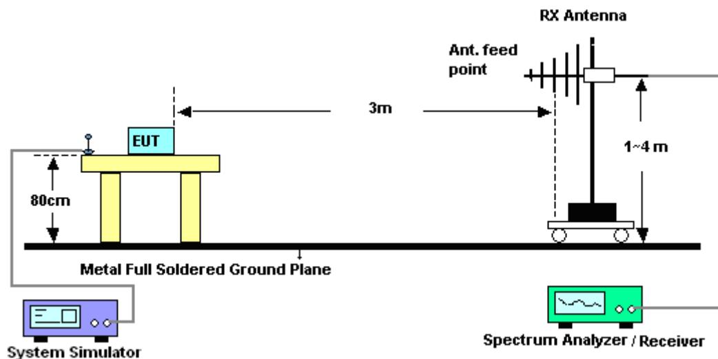
For radiated test above 1GHz
