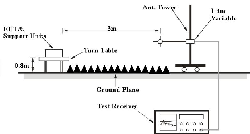
The radiated emission tests were performed at the 3 meters distance in chamber, using the setup accordance with the ANSI C63.4-2014. The specification used was the FCC Part 15.109 Class B limits.
