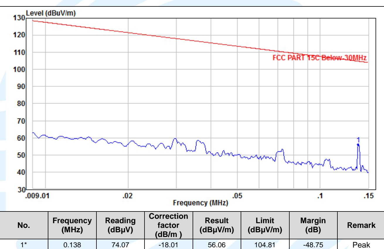
**Radiated Emission Test Data (150 KHz ~ 30 MHz):**
