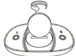
**B.** Remove the old battery and insert the new battery with the +side upwards.
