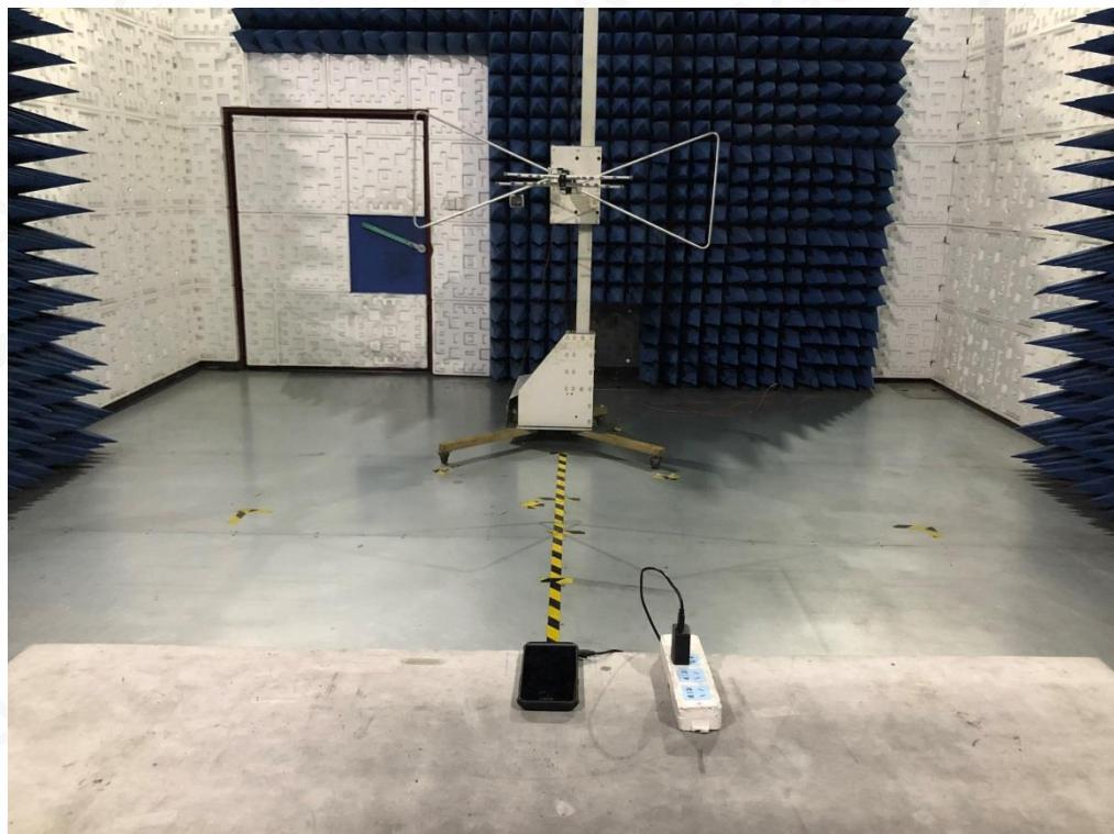
**FCC RADIATED EMISSION TEST SETUP ABOVE 1GHZ**
