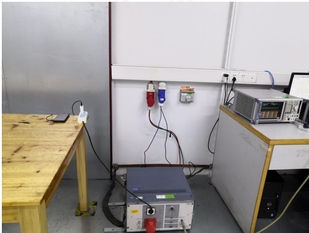
RADIATED EMISSION TEST SETUP BELOW 30MHz
