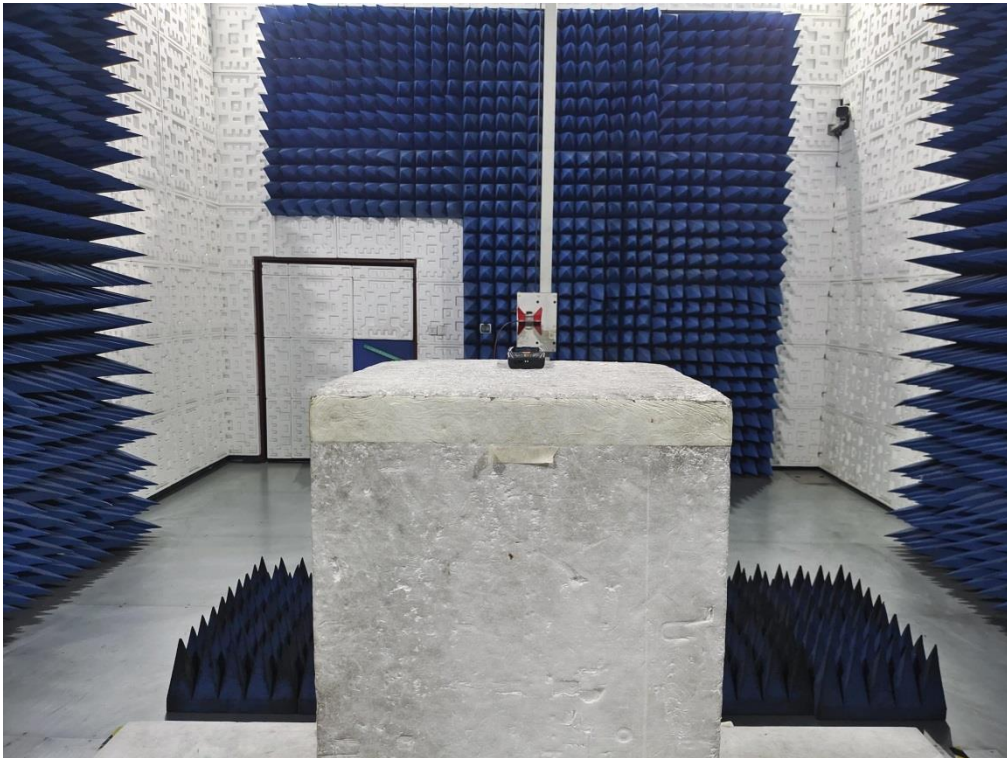
FCC RADIATED EMISSION TEST SETUP ABOVE 1GHZ
