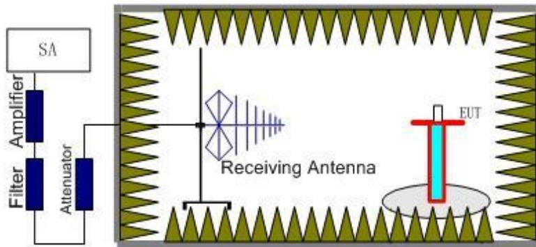
Radiated emissions measurements were made only at the upper, middle, and lower carrier frequencies of the LTE band 2, the LTE band 4 and LTE band 17. It was decided that measurements at these three carrier frequencies would be sufficient to demonstrate compliance with emissions limits because it was seen that all the significant spurs occur well outside the band and no radiation was seen from a carrier in one block of any band into any of the other blocks.
