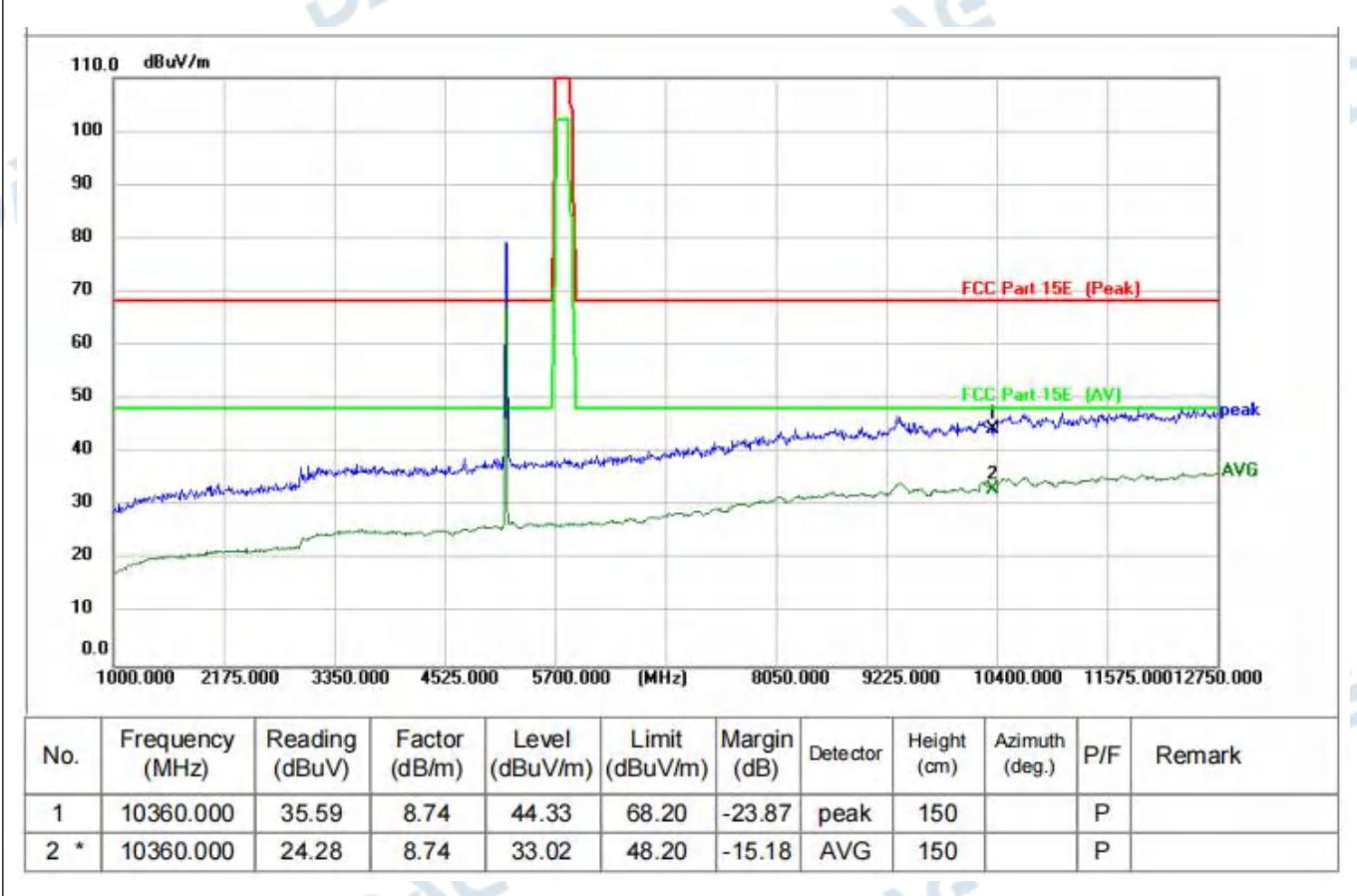
TM1 / Polarization: Vertical / Band: 5150-5250 MHz / BW: 20 / CH: L
