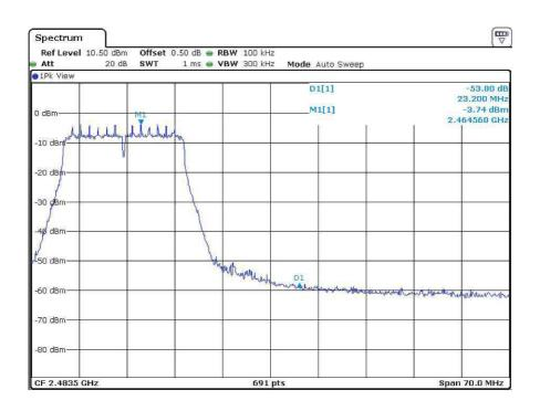
802.11n-HT40 Channel 01 (2422MHz) Reference Level: -5.60dBm
