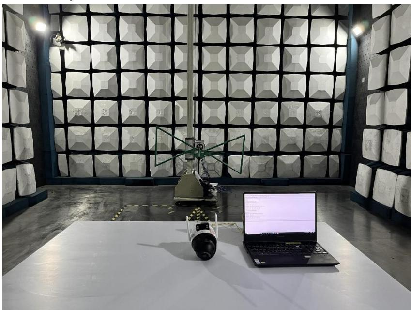
**Radiated Spurious Emissions Above 1GHz**
