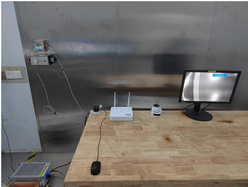
Conducted Emissions at AC Power Line (150kHz-30MHz)
