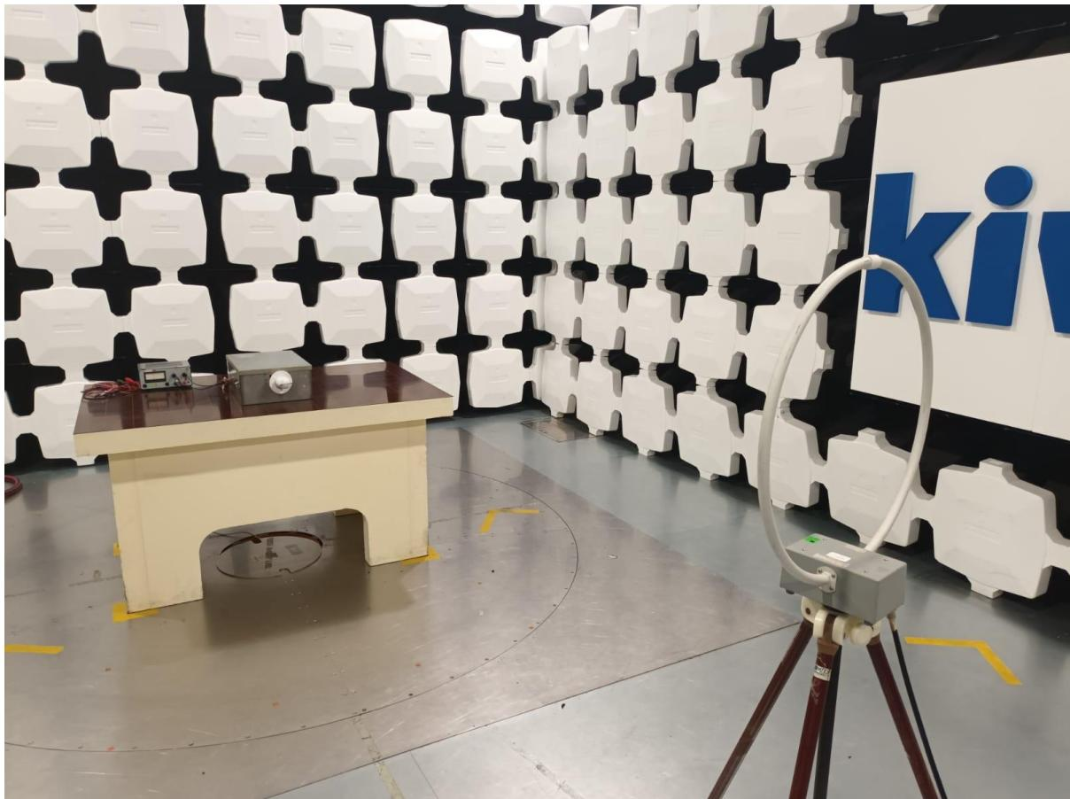
Note: The grey box on the test table is a host for the EUT prepare by the customer for the testing.
