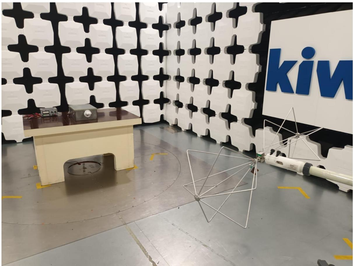
Note: The grey box on the test table is a host for the EUT prepared by the customer for the testing.
