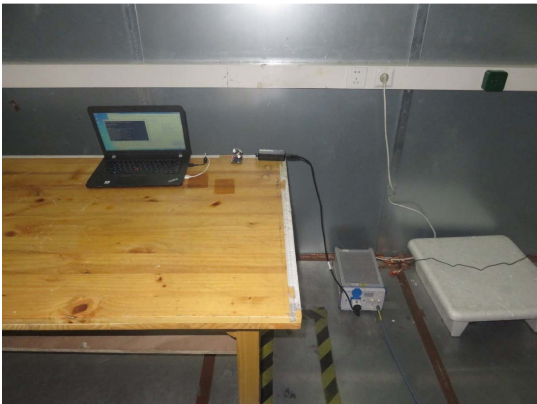
Picture 3 Conducted Emission Test Setup
