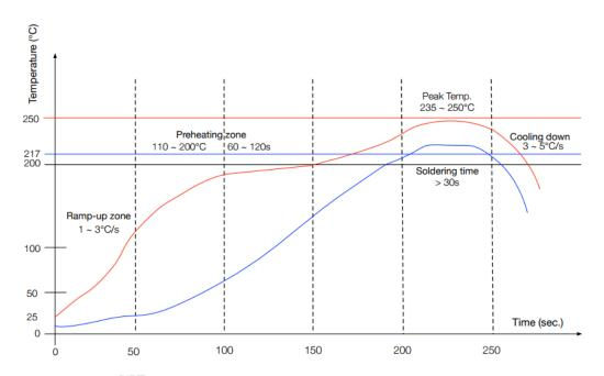
Ramp-up zone (升温区): Temp. <150°C, Time  $60\sim90$ s, Ramp-up rate  $1\sim3$ °C/s. Preheating zone (预热恒温区): Temp. 150  $\sim200$ °C, Time  $60\sim120$ s, Ramp-up rate  $0.3\sim0.8$ °C/s. Reflow soldering zone (回流焊接区): Peak Temp. 235  $\sim250$ °C ( <245°C recommended), Time  $30\sim70$ s. Cooling down zone (冷却区): Temp. 217  $\sim170$ °C, Ramp-down rate  $3\sim5$ °C/s. Sn&Ag&Cu Lead-free solder (SAC305)/焊料为锡银铜合金无铅焊料
